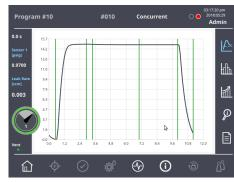
The reimagined touchscreen provides access to a wide range of data. From statistics like pass, fail, minimum, maximum, and standard deviations, to historical graphs and charts, the Sprint<sup>mD</sup> provides a deep level of information, making it easy to monitor the process.
